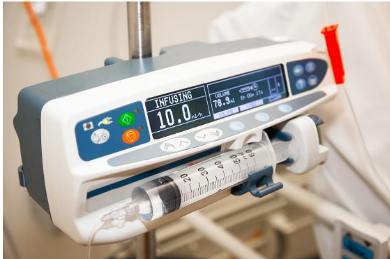
The plunger of the syringe is pushed forward by the pump at the programmed rate
